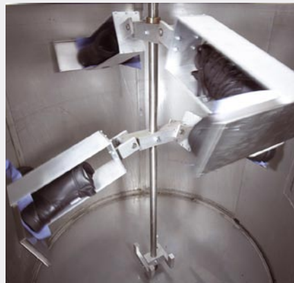
Gore boots being tested for waterproofing, taking 300,000 steps through water and flexing in the Gore laboratory
