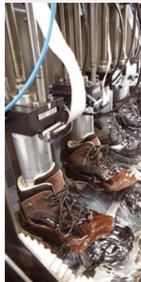
Gore boots being tested for waterproofing, taking 300,000 steps through water and flexing in the Gore laboratory
