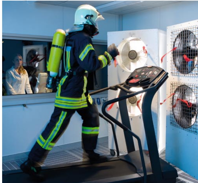
Gore product testing involves a variety of simulated environments – including heat and wind – to ensure garments perform well for the emergency services
