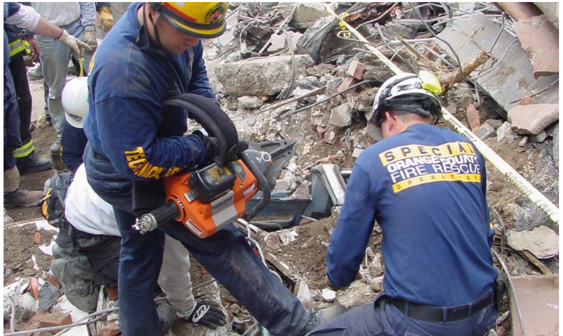
Compact and lightweight, battery-powered extrication tools are much more versatile, owing to their portability
